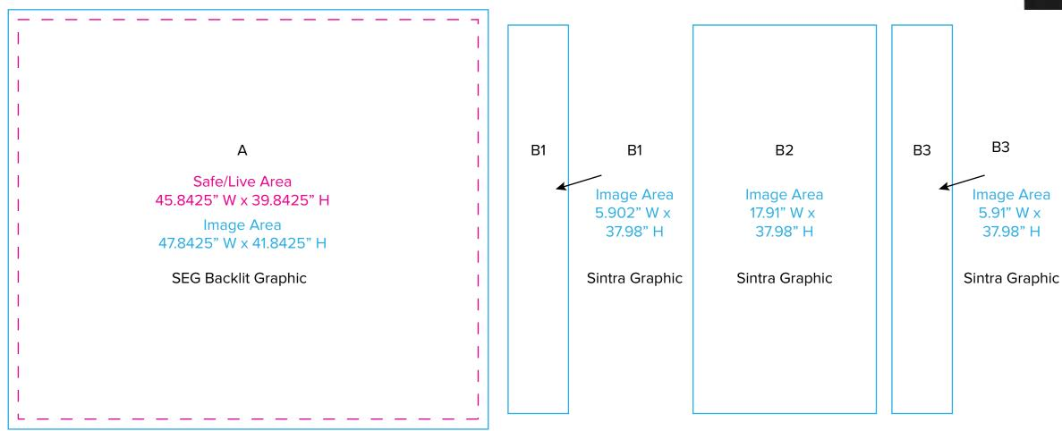
Sintra Note: 1/4" of graphic perimeter is hidden by extrusion
